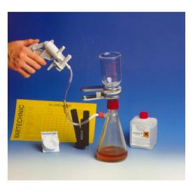
With the help of a micro magnifyinglens it is possible to determine quantity, dimensions and even the origin of impurities! Abrasions on pistons, pumps, etc. may be detected in time to react before results become catastrophic.
